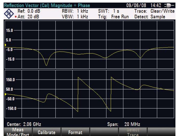
FIG 2 Simultaneous display of magnitude and phase in split-screen mode.
